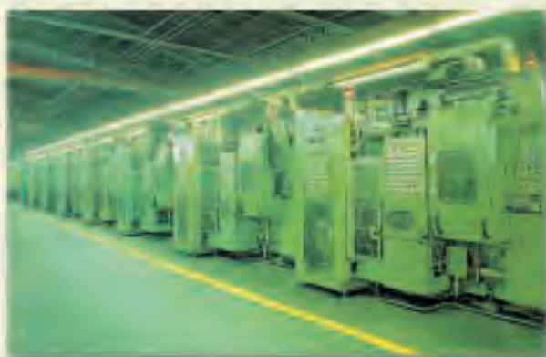
Grinding process of outer rings 外圈研磨工序
